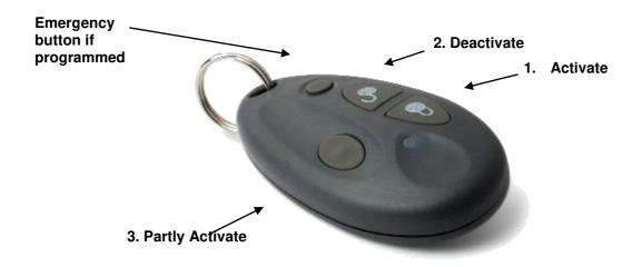
$\underline{\text{Note:}}$  The buttons on the wireless key fob are sensitive. Kindly handle the fobs with care to avoid false alarms.
